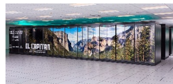
El Capitan 2.7 Eflop/s, 30MW 43k 24-core CPUs + 43k GPUs #1 in Top500
