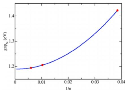
Fig. 1. Computed gap (in eV) of silicon (1.422 eV, 1.21 eV, and 1.20 eV corresponding to 26, 97, and 168 bands with red dots representing the raw data) versus the inverse of the number of bands.
